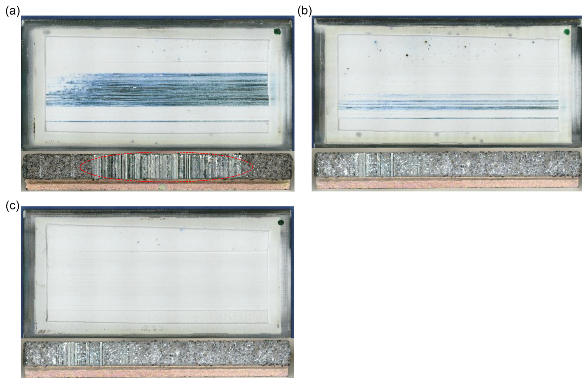
FIGURE 5 | Images of (a) liner (i), (b) liner (ii), and (c) liner (iii) after incursion test, at the bottom of each image the cut-in blades are shown; the dark blue color of liner (i) and liner (ii) indicate material transfer from the blade; liner (iii) presents the best incursion test results.
